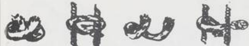
154. Form of the knots of the Guerdès carpets, Turkey 155. Different ways of fastening the knots
